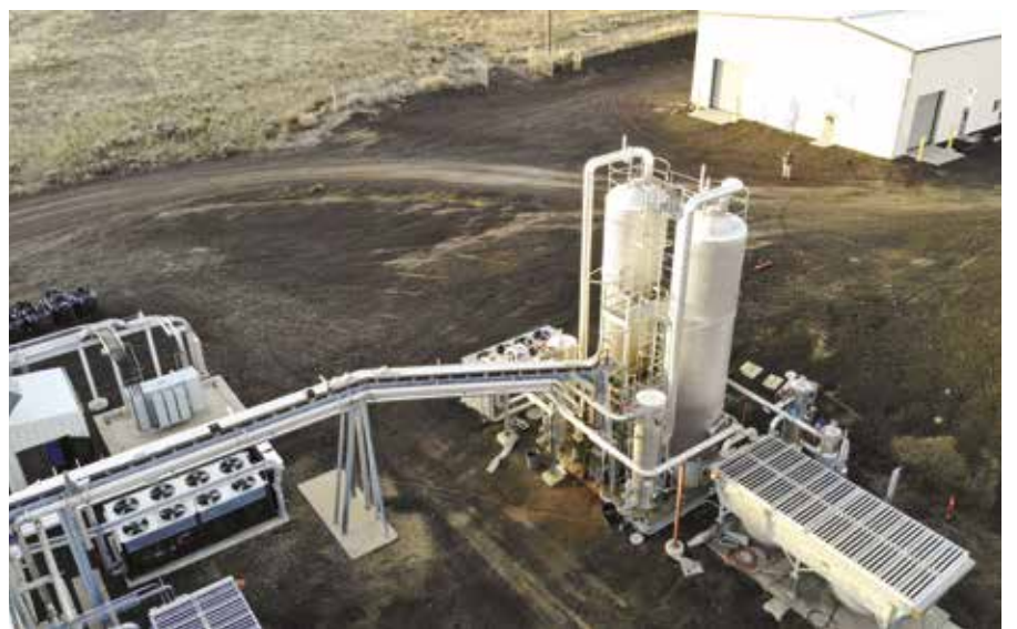
Chelated iron system for scrubbing biogas at a project site in Washington.
