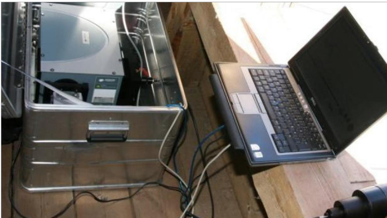
**Figure 5.** The FluxSense SkyDOAS system consisting of a telescope, optical fiber, spectrometer, and control computer (Mellqvist et al., 2017).
