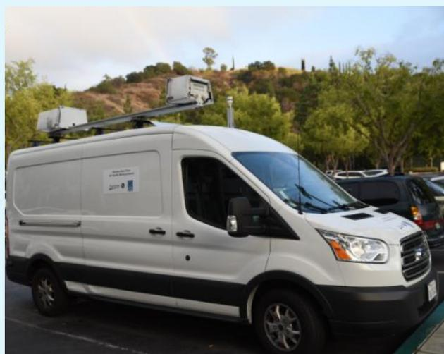
**Figure 2.** View of MWDOAS instrument mounted atop the FluxSense mobile laboratory (Mellqvist et al., 2017).
