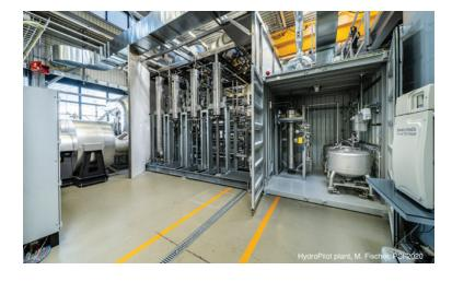
TreaTech's patented technology uses hydrothermal gasification (HTG) to convert waste streams that are usually incinerated into integral products, such as clean water for industrial and consumer use, minerals including phosphorous, nitrogen and potassium used for fertilizer, and crucially a constant supply of methane-rich renewable gas that can be used as an onsite energy solution or injected into the grid network.
